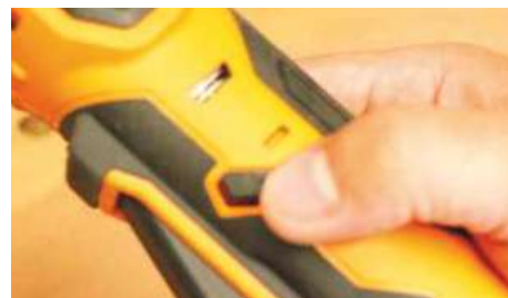
▲ The tool is very basic, having only a forward/reverse button and variable-speed trigger
